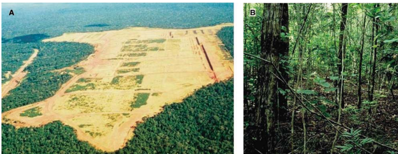
Fig. 3. (A) An aerial view of the open-cut bauxite mine at Trombetas in central Amazonia that is located in a relatively undisturbed area of evergreen equatorial moist forest. A reforestation program treats about 100 ha of mined land per year by using stockpiled topsoil and by planting a variety of native species with direct seeding, stumped saplings, or potted seedlings. (B) Within 10 years of establishment, most sites have many more tree and shrub species than the number initially planted because of seed stored in the topsoil or colonization from the surrounding forest. These new species would have been brought to the site by birds, bats, and terrestrial mammals, and most were species with small seeds. Overall it seems the reforestation program has been successful in facilitating the reestablishment of both plants and animals to the site, although more time will be needed for the composition and structure to closely resemble nearby intact forest (SOM Text).
